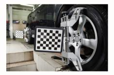
On newer cars with AI, any service that requires an alignment also may require an ADAS calibration. Even the slightest misalignment in the cars 4-wheel alignment can cause the cars ADAS to not function property, and potential for being the cause of an accident.
